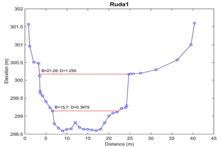
**Figure 2. Example plot of a channel cross-section from a local survey for the Ruda River in Croatia.**
