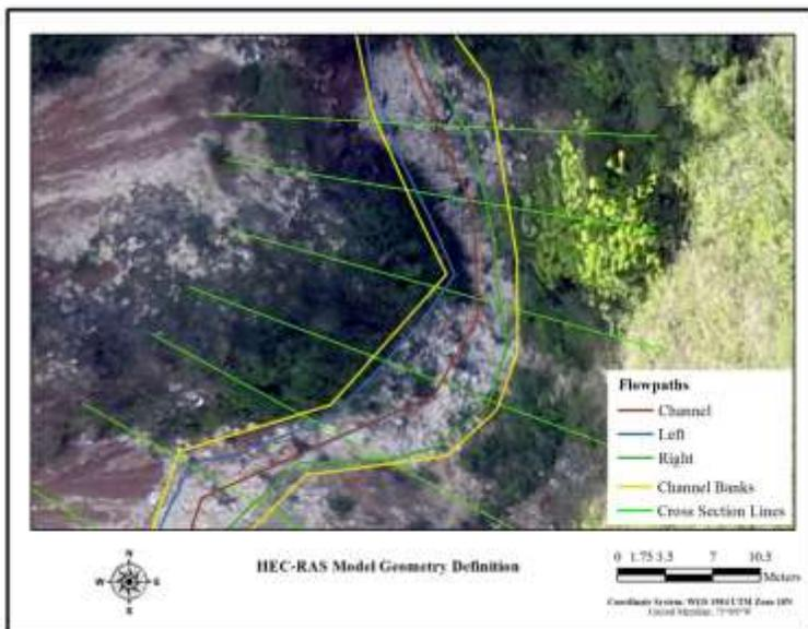
Figure 1. Hi-resolution numerical representations of the watershed and channel geometries.
